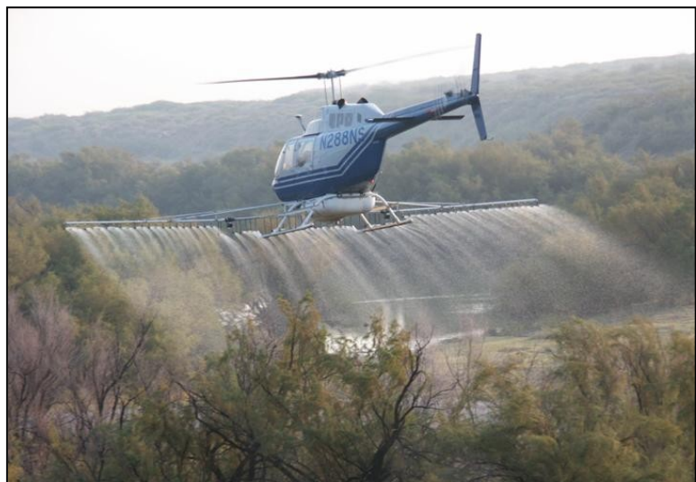
Use of helicopters to apply herbicide provides the convenience of aerial application with the added benefits of allowing precision application, virtually eliminating chemical drift, and allowing the landowner to selectively treat very specific areas.
