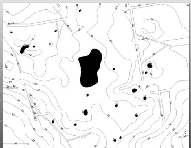
Figure 2: A subsection of the 1919 Cedar Bayou vector data with the contours annotated and the depressions selected and highlighted in black.
