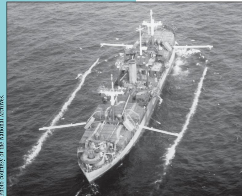
*Liberty Ship steaming with anti-torpedo nets deployed.*
