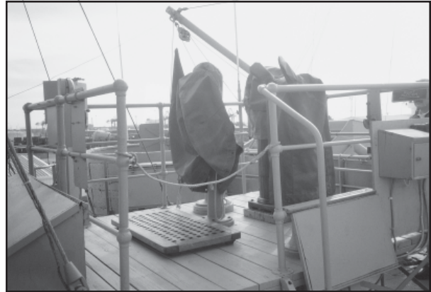
Figure 14. Topside conning station located above the wheelhouse on the John W. Brown . In fair weather the Liberty Ships were usually steered from this position since the view from the wheelhouse is very restricted (Photo by Barto Arnold 1995).
