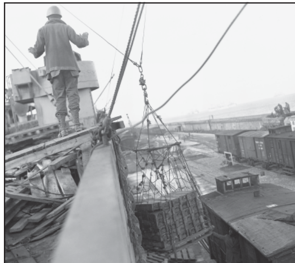
Figure 21. At a French port ammunition receives priority handling from Liberty Ship to railway box car for quick dispatch to the front. Off loading by pallets as shown permits the handling of 30 boxes at one time, containing 60 projectiles for the 105-mm howitzer, the backbone of the US field artillery, Nov. 4, 1944 (National Archives).
