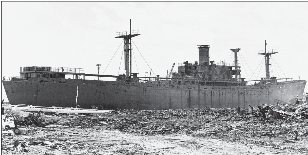
Figure 40. One of the twelve Liberty Ships awaiting the cutting touch at Andy International, Incorporated's ship breaking yard in Brownsville, Texas. The ships were cut down for sinking to serve as artificial reefs in a program carried out by the Texas Coastal and Marine Council in 1975-76 (Texas Coastal and Marine Council 1975).
