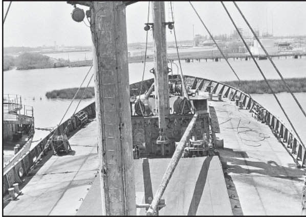
Figure 41. The super structure and all masts and posts were removed from the Liberty Ships (Texas Coastal and Marine Council 1975).
