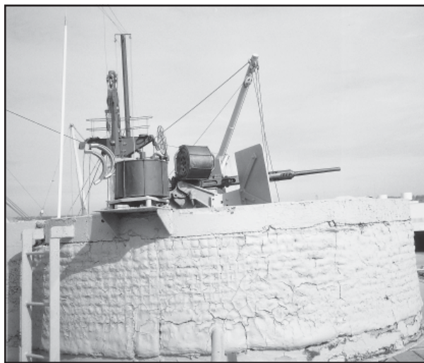
Figure 17. Twenty-mm gun on the John W. Brown . Note the so-called plastic armor on the outside of the gun tub (Photo by Barto Arnold 1995).
