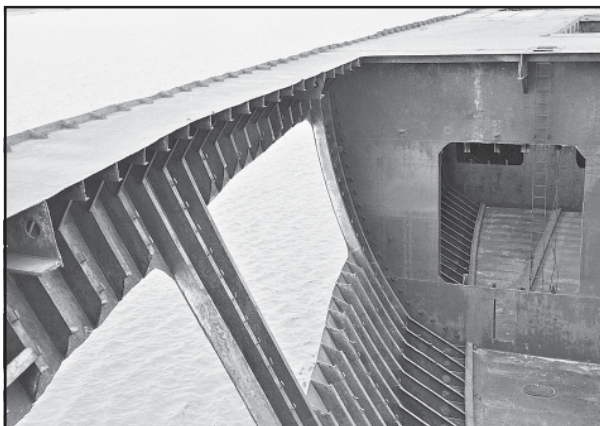
Figure 48. Inside view of a cleaned Liberty Ship that is ready for sinking. Note holes in left side to allow for water circulation. (Texas Coastal and Marine Council 1975).
