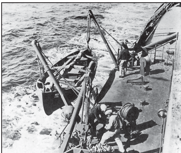
Figure 10. Testing the davits for launching a boat on a Liberty Ship (Douglas and Salz 1943).
