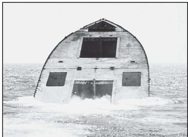
Figure 51. With the stern already resting on the bottom, the bow of this Liberty Ship submerged to form a part of an artificial reef (Texas Coastal and Marine Council 1975).
