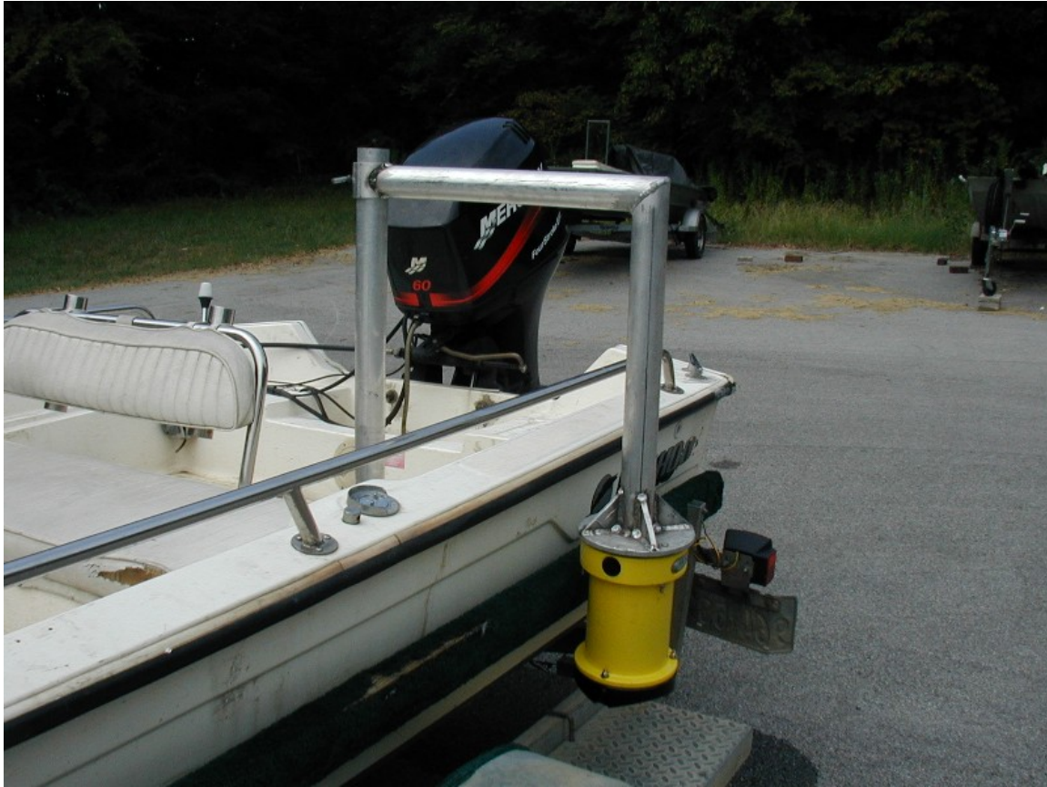
Figure 6.—Boat-mounted River Surveyor (ADCP) configuration that was used to collect flow data on Cow Bayou and Lost River beginning with the August 2003 trip.
