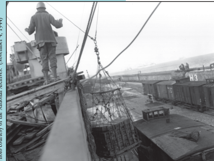
At a French port ammunition receives priority handling from Liberty ship to railway box car for quick dispatch to the front. Off loading by pallets permitted the handling of 30 boxes at one time, with each box containing 60 projectiles for the 105 mm howitzer, the backbone of the U.S. field artillery.
