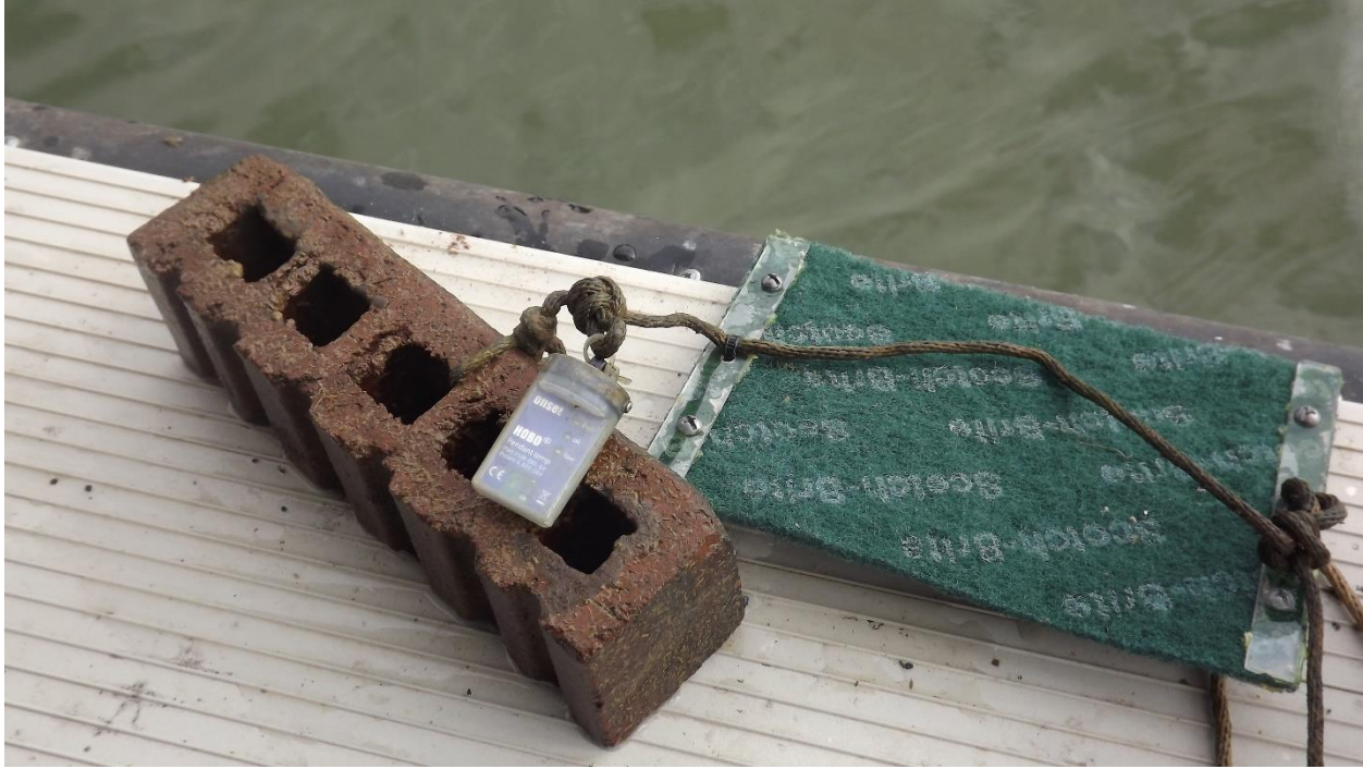
Figure 8. Nylon scrub pad juvenile mussel settlement monitor fixed to lopes in a house-brick weighted nylon rope with plastic electrical ties. Also note attachment of an Onset™ Hobo temperature data logger fixed to a loop in the rope with a plastic electrical tie.
