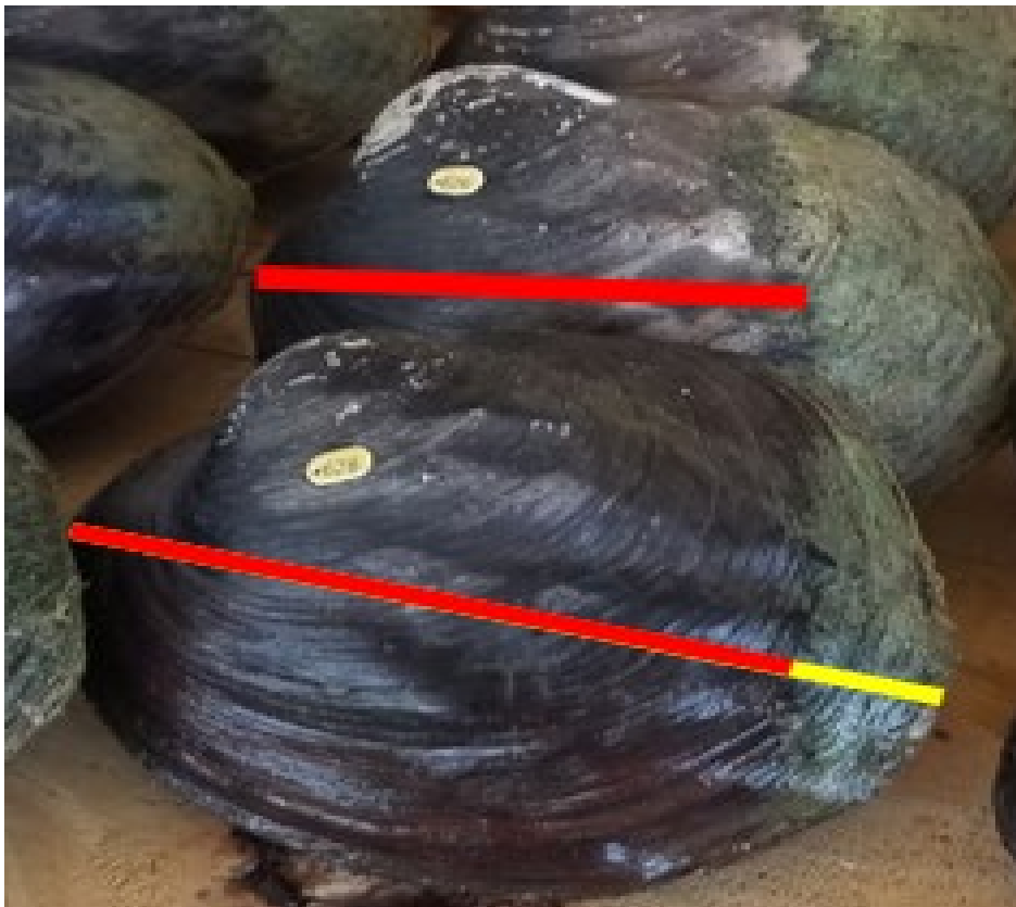
Figure A1: Technique for measuring unionid mussel burrowing depth. The yellow line indicates total mussel shell length while the red line indicates total mussel burrowing depth.
