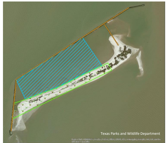
Conceptual drawing of the Smith Point Island restoration, illustrating the breakwater, fill, and emergent shell substrate area
