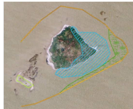
Conceptual drawing of the Dressing Point Island restoration, illustrating the breakwater, fill, shell knoll, and potential marsh restoration
