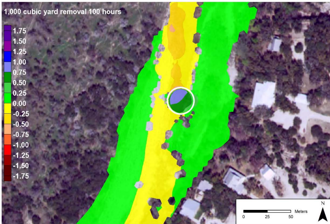
FIGURE G51.—Sediment deposition after 100 hours of simulation (in meters), 1000 cubic yards of material removed from the river at the middle site. The white circle denotes the location where material was removed.
