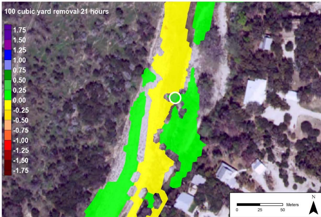
FIGURE G19.— Sediment deposition after 21 hours of simulation (in meters), 100 cubic yards of material removed from the river at the middle site. The white circle denotes the location where material was removed.
