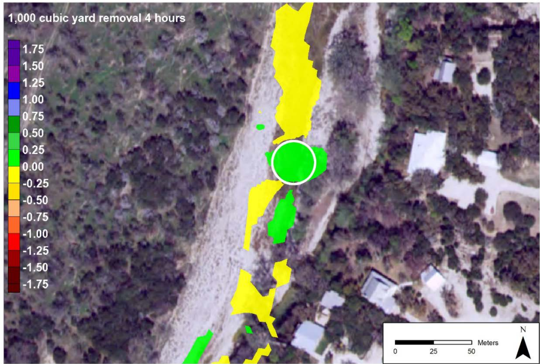
FIGURE G12.—Sediment deposition after 4 hours of simulation (in meters), 1000 cubic yards of material removed from the river at the middle site. The white circle denotes the location where material was removed.
