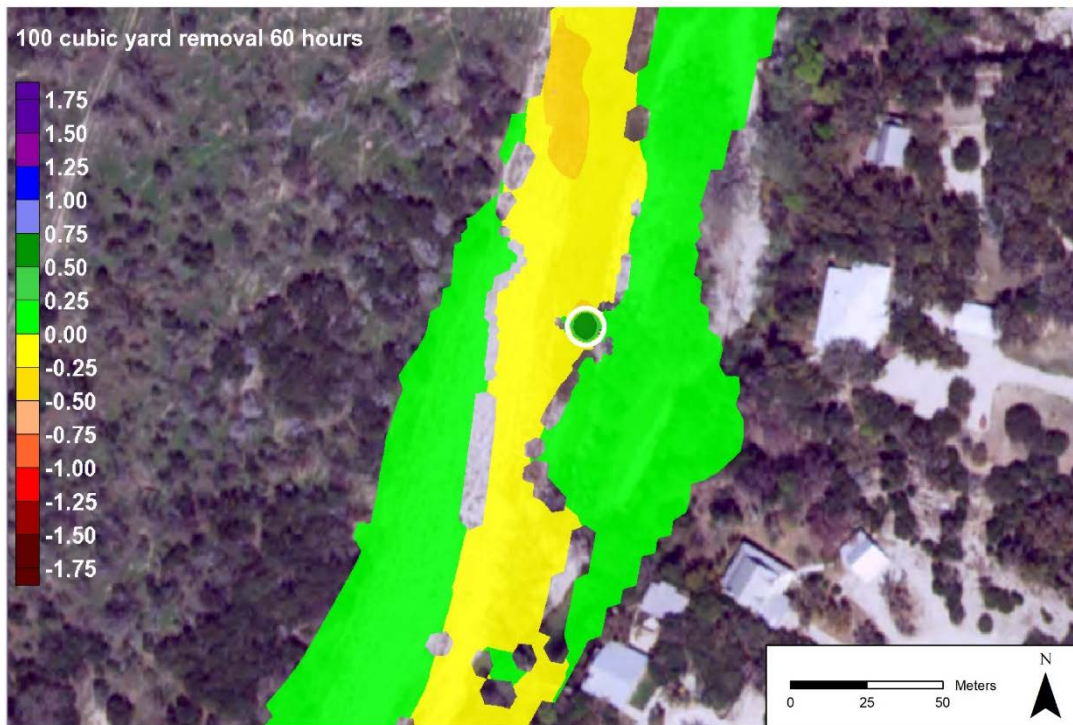
FIGURE G32.—Sediment deposition after 60 hours of simulation (in meters), 100 cubic yards of material removed from the river at the middle site. The white circle denotes the location where material was removed.
