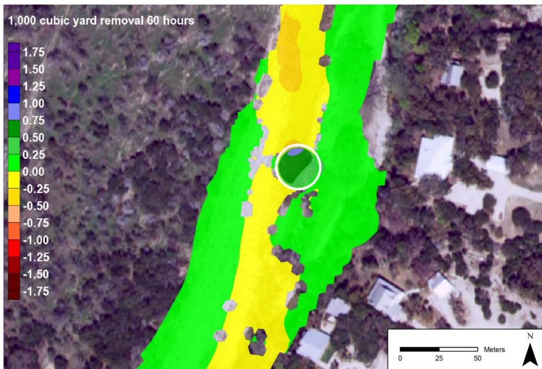
FIGURE G38.—Sediment deposition after 60 hours of simulation (in meters), 1000 cubic yards of material removed from the river at the middle site. The white circle denotes the location where material was removed.
