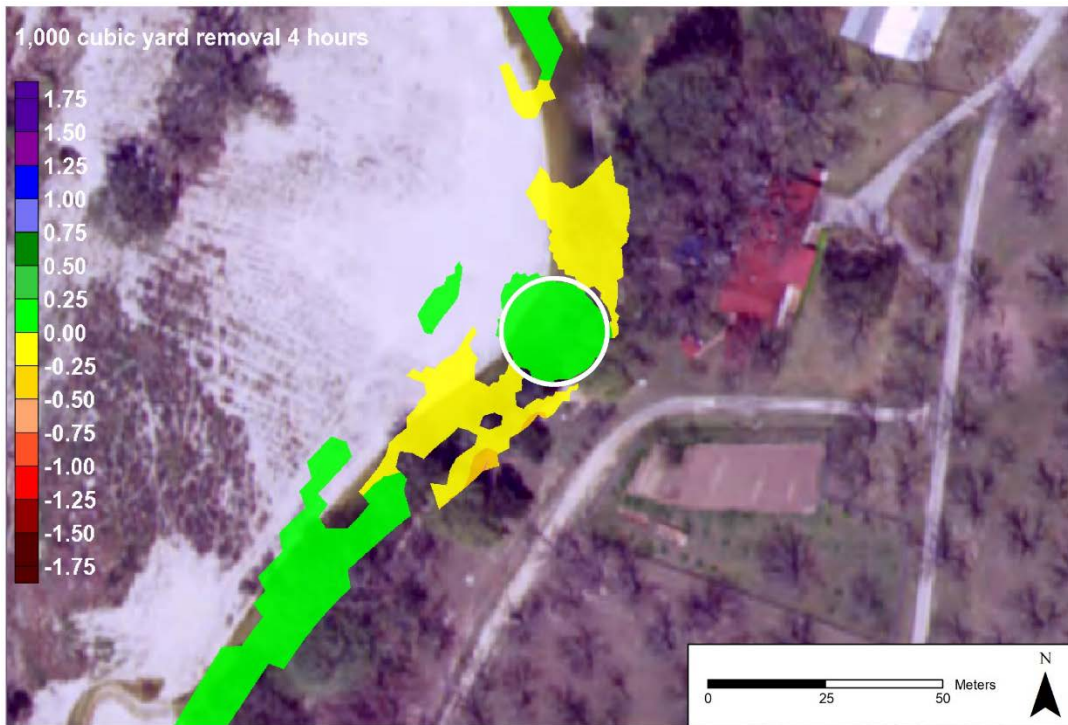
FIGURE G13.—Sediment deposition after 4 hours of simulation (in meters), 1000 cubic yards of material removed from the river at the lower site. The white circle denotes the location where material was removed.
