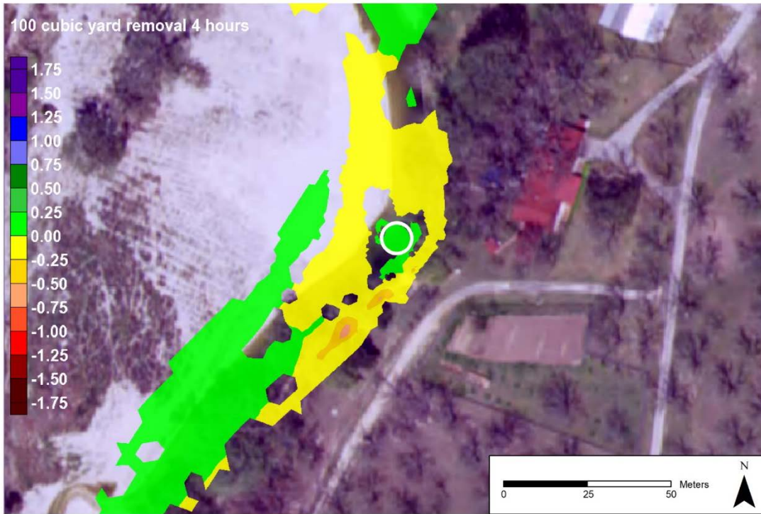
FIGURE G7.—Sediment deposition after 4 hours of simulation (in meters), 100 cubic yards of material removed from the river at the lower site. The white circle denotes the location where material was removed.
