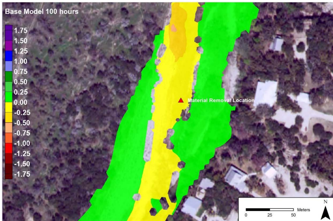
FIGURE G42.—Sediment deposition after 100 hours of simulation for the base sediment model run (in meters) with no material removed from the river. The red triangle denotes the location where material removal will occur in later model runs (middle site).
