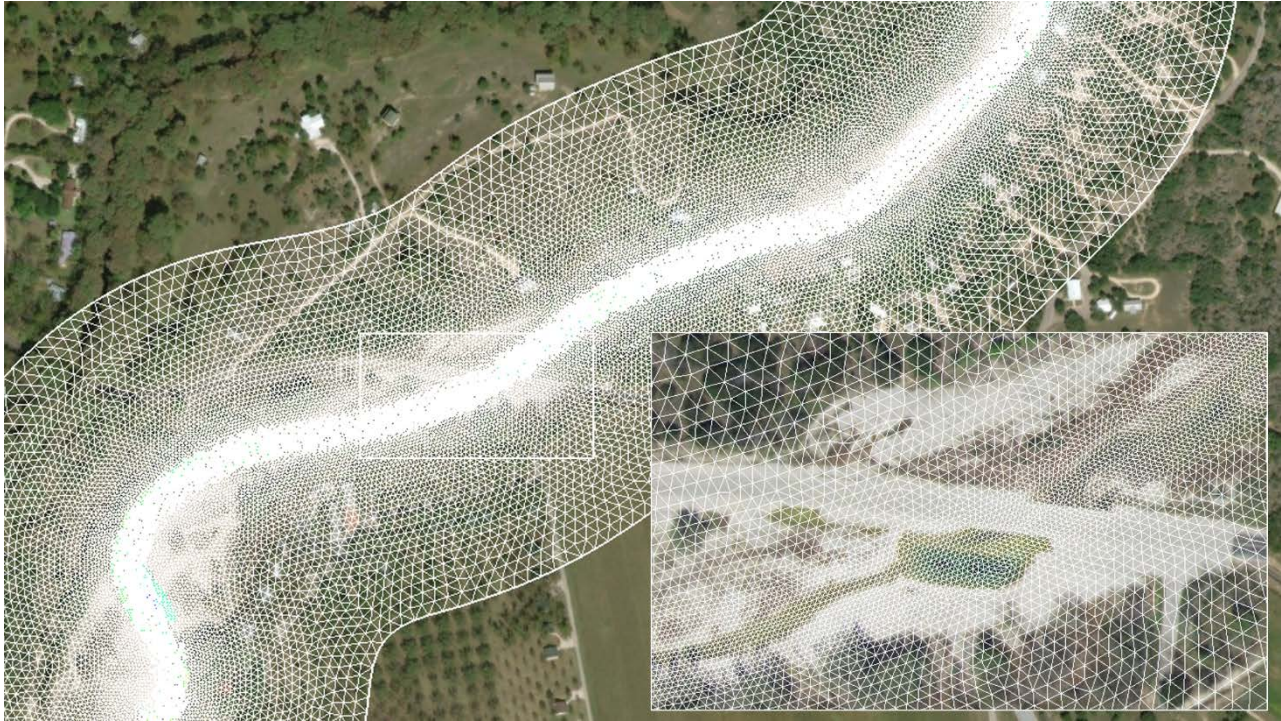
FIGURE F10.—AdH mesh on the Frio River near Leakey, Texas. Notice the greater number of computation nodes and elements closer to the center of the channel for higher resolution.
