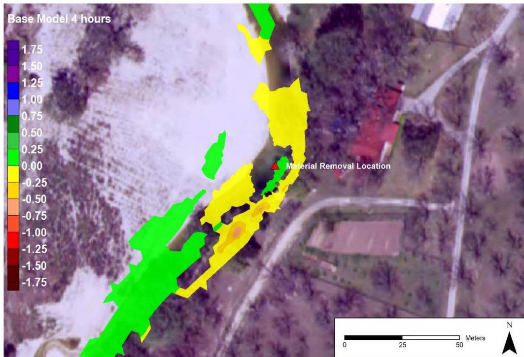
FIGURE G4.—Sediment deposition after 4 hours of simulation for the base sediment model run (in meters) with no material removed from the river. The red triangle denotes the location where material removal will occur in later model runs (lower site).
