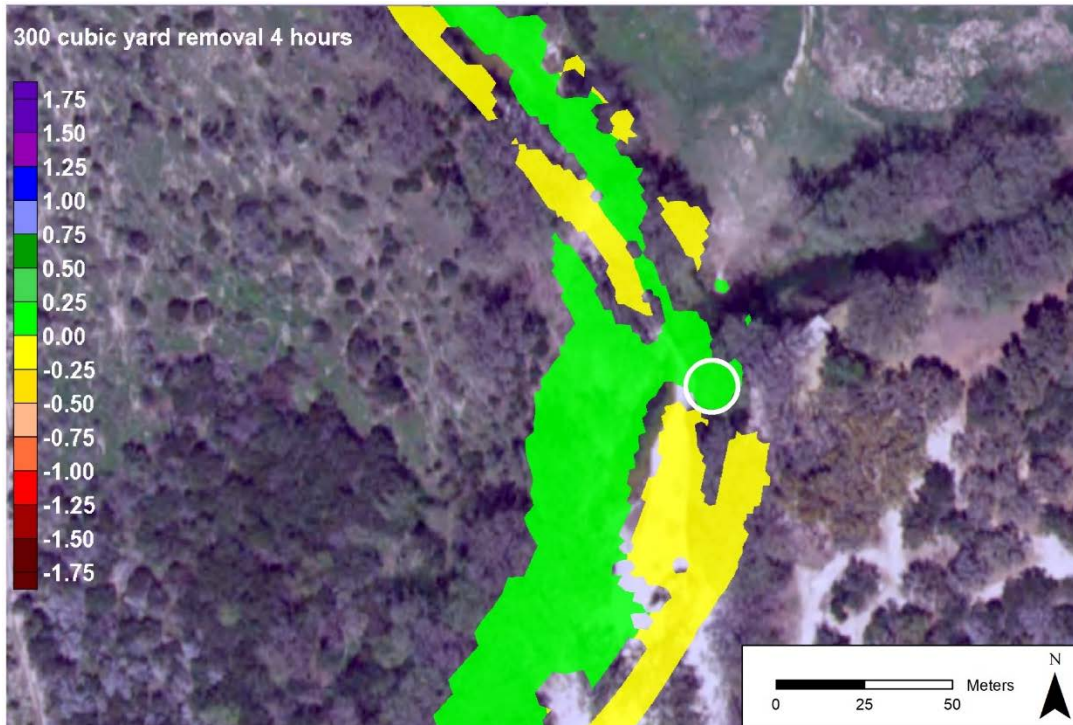
FIGURE G8.—Sediment deposition after 4 hours of simulation (in meters), 300 cubic yards of material removed from the river at the upper site. The white circle denotes the location where material was removed.
