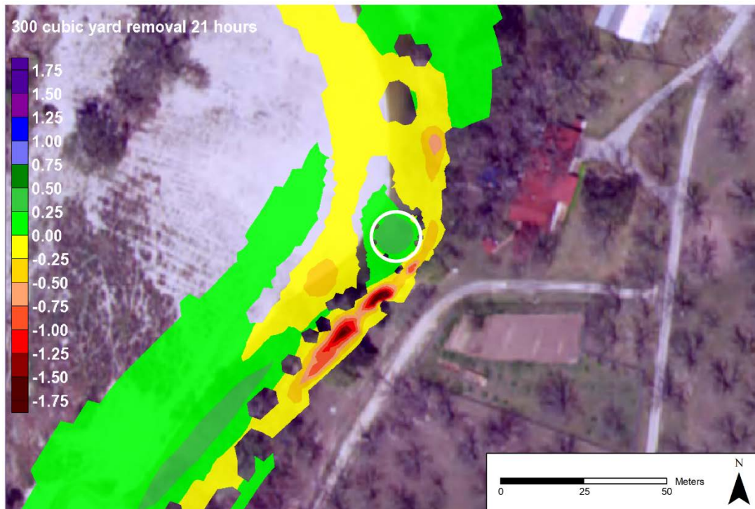
FIGURE G23.—Sediment deposition after 21 hours of simulation (in meters), 300 cubic yards of material removed from the river at the lower site. The white circle denotes the location where material was removed.
