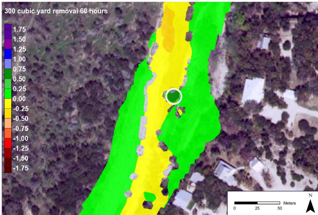
FIGURE G35.—Sediment deposition after 60 hours of simulation (in meters), 300 cubic yards of material removed from the river at the middle site. The white circle denotes the location where material was removed.
