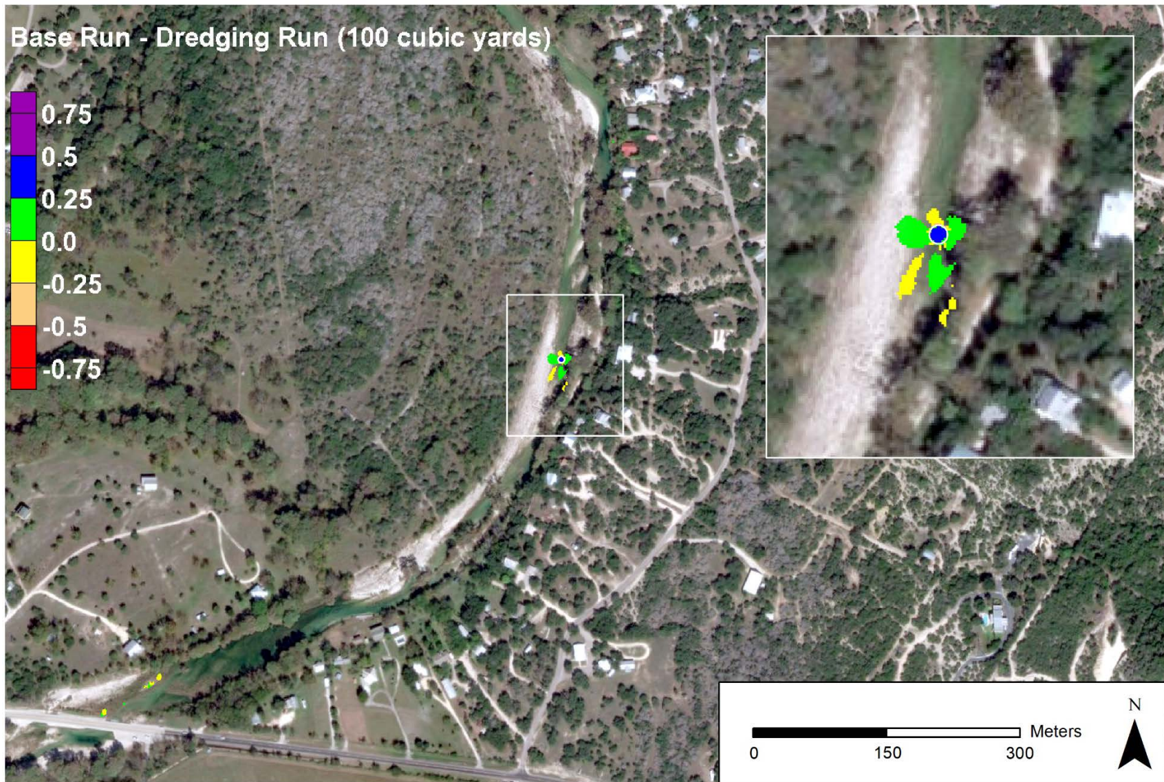
FIGURE F24.—This map shows the amount of change in deposition (relative to the base sediment model run, in meters) following removal of 100 cubic yards of material. Note the material removal site by the white circle.
