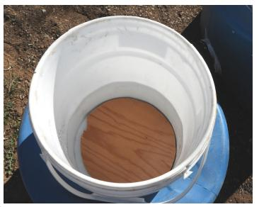
Insert the bucket into the top hole and the short sections of drainage pipe into the side holes of the barrel.
